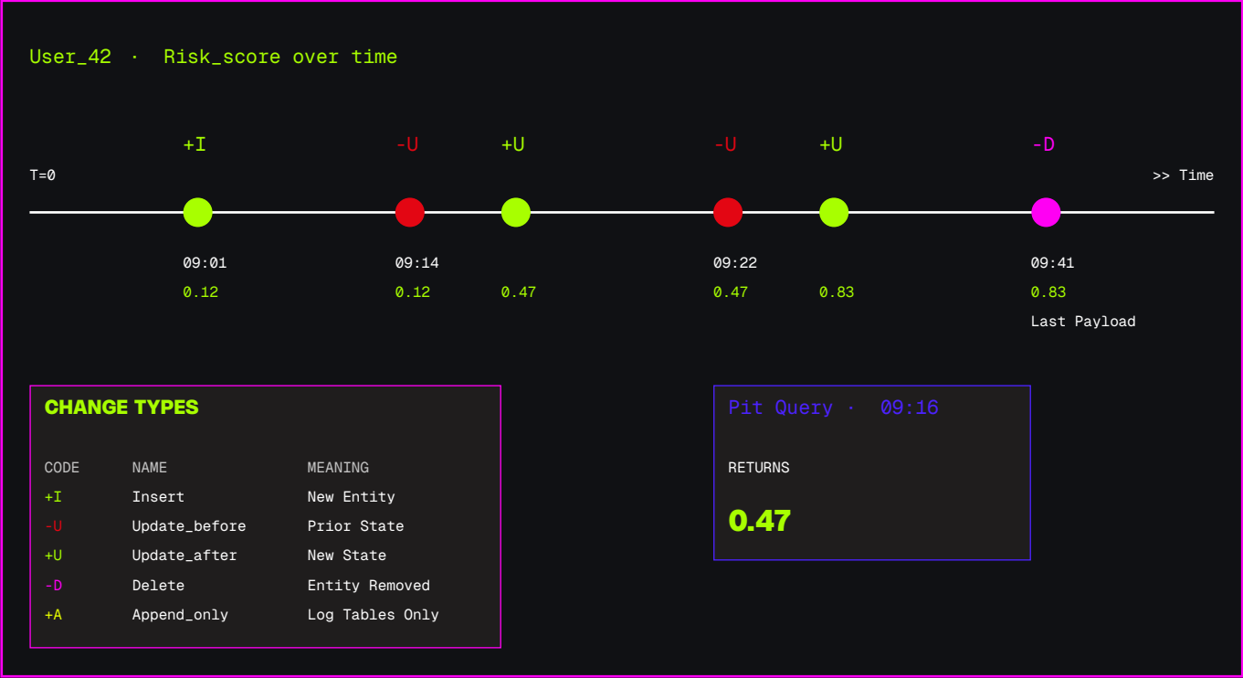
DIAGRAM 8: CHANGELOG SEMANTICS Every PK Table update produces a -U / +U pair. Every delete emits a -D record carrying the last known row payload, downstream consumers reconstruct the deleted state from the -D itself. This enables point-in-time correct reads across the entire history.
